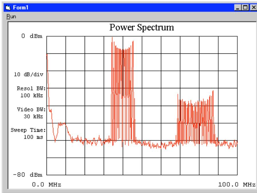
Figure 2: Typical heterodyne signal
