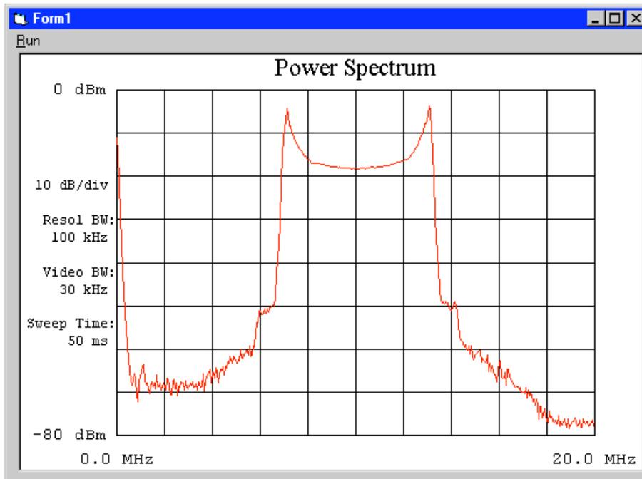
Figure 3: Simulated heterodyne signal
