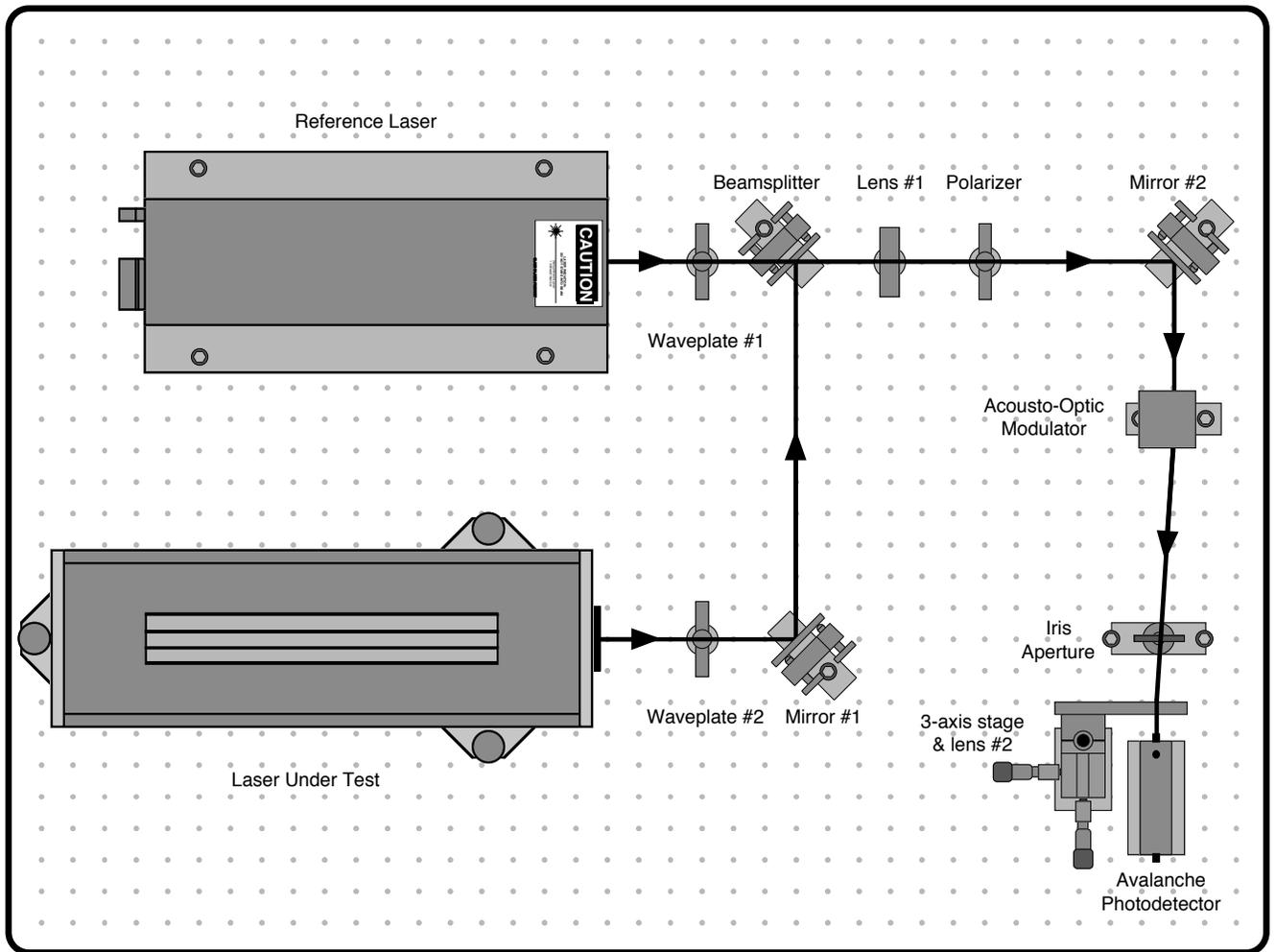
Figure 1: Optical Heterodyne Setup
